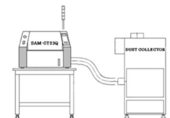
**3** Dust Collection from underside of cutting JIG, thus minimized adhesion of dust.
