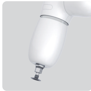
Electric Vacuum Generator*3
